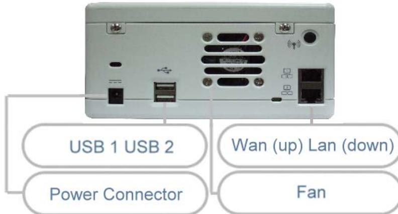
The rear panel of the N299 houses the USB and Ethernet connections, as well as the power connector. See the table below for descriptions of each:
