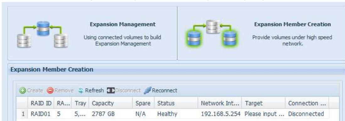
Our sample unit 2 is WAN/LAN1 IP 172.16.66.111, 10G NIC IP 192.168.5.250 and the volume used for volume expansion is created in RAID10.
