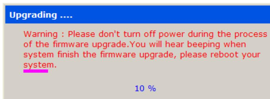
**NOTE: During firmware upgrade process, it is imperative that user do not turn off the power to N4100Plus or close the browser. This will lead to catastrophic result.**
